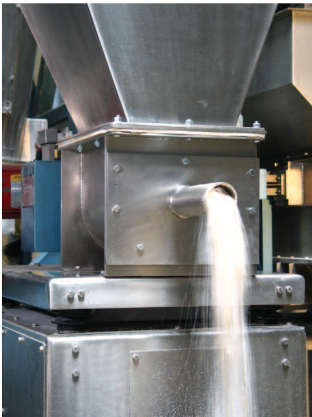
Tests conducted by the feeder supplier demonstrate this gravimetric feeder's ability to accurately feed an additive for a customer's plastics compounding operation.
