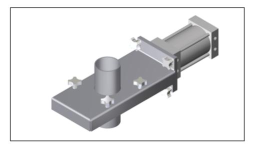
The standard gate is constructed from 304 Stainless Steel (Body components, Inlet and Outlet stub and Blade) and utilizes UHMW pressure plates. 316 Stainless Steel construction is also available.
