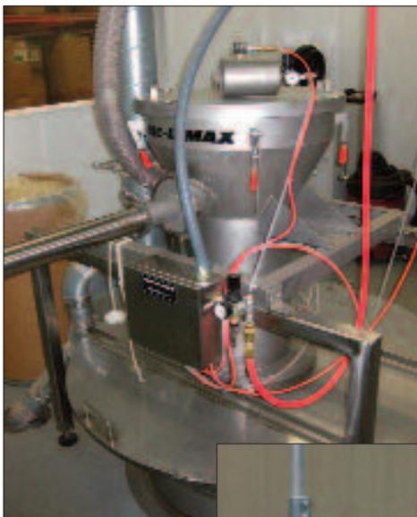
Pneumatic conveying systems have many advantages over open conveying systems such as belt or bucket conveyors. Ease of cleaning and the smaller footprint of pneumatic conveying systems are two of its biggest advantages.
