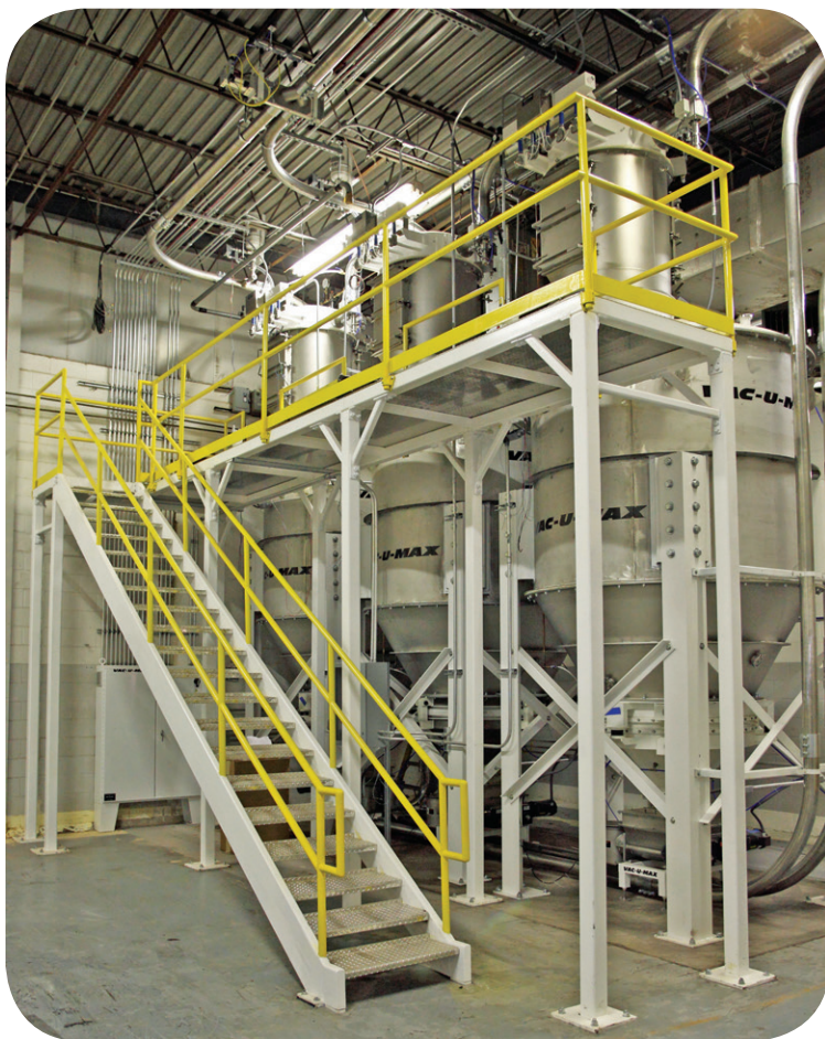
These 300-cu-ft material receivers are part of a pneumatic conveying system that transfers powders in a large-scale candy making process.
