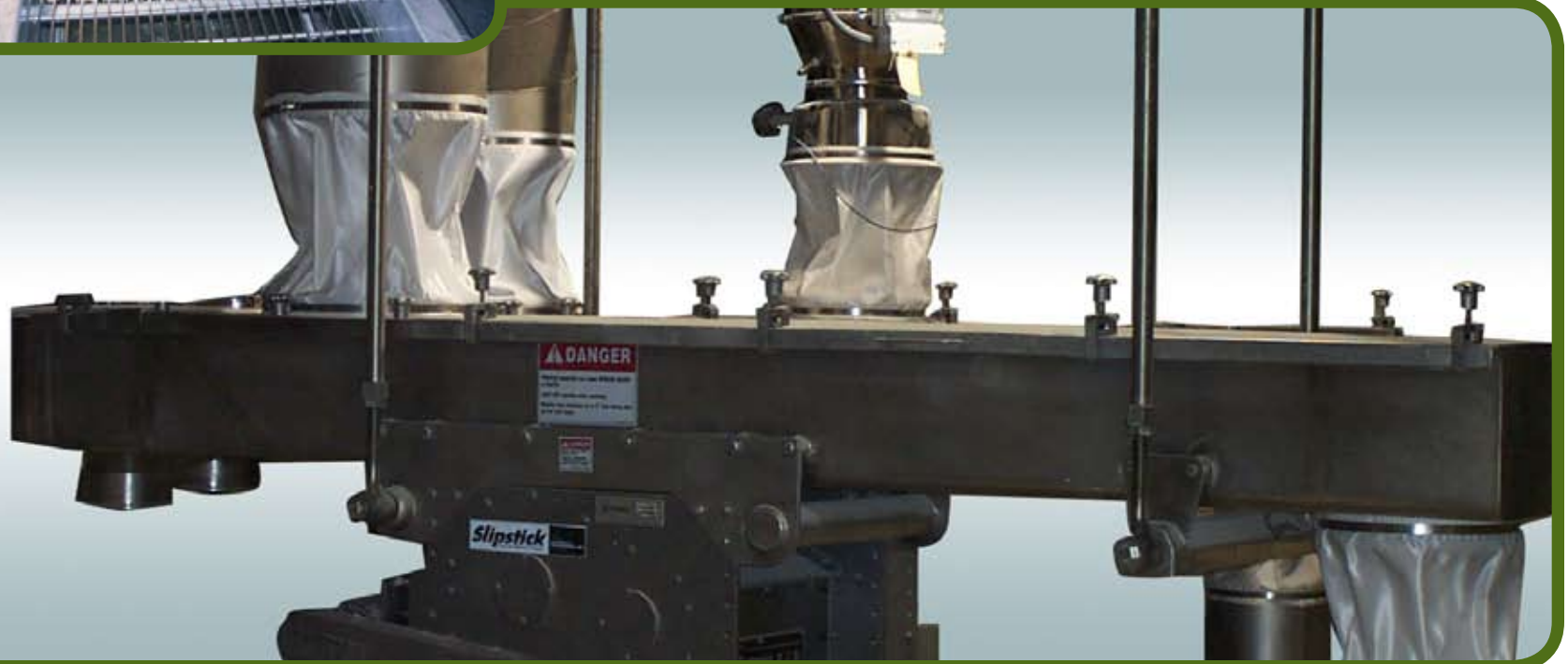
Sealed inlets and outlets may be used for dusty products.
