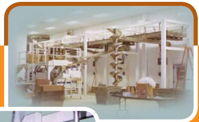
Support structures such as access platforms and walkways may be included to tie together multiple conveyors or to support other equipment.
