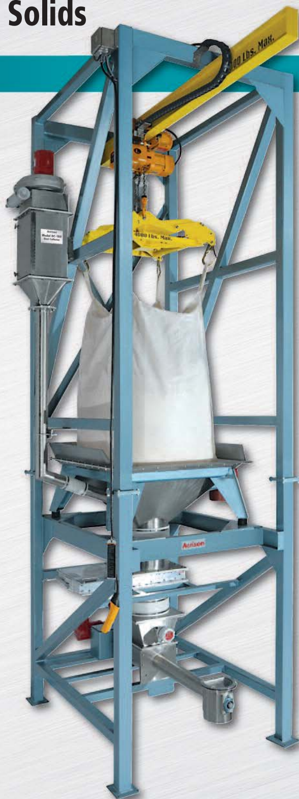
A Model 810 Bulk Bag Unloader mounted above an Acrison Volumetric Feeder (a maintenance gate is provided between the Bulk Bag Unloader and the feeder). The Bulk Bag Unloader also includes an electric hoist and motorized trolley, Acrison's Automatic Tensioning Bag Lifting Rack and Dust Collector.
