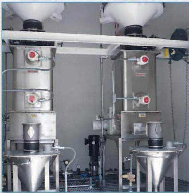
Two Model BDF-1.5 Volumetric Feeders, each feeding powdered activated carbon into an Acrison high-capacity wetting cone .
