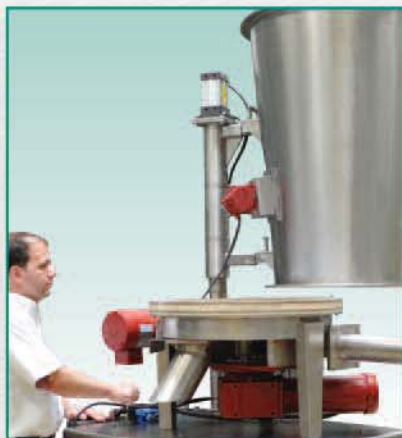
Pneumatically operated Swing-Out Hopper (certain models)
