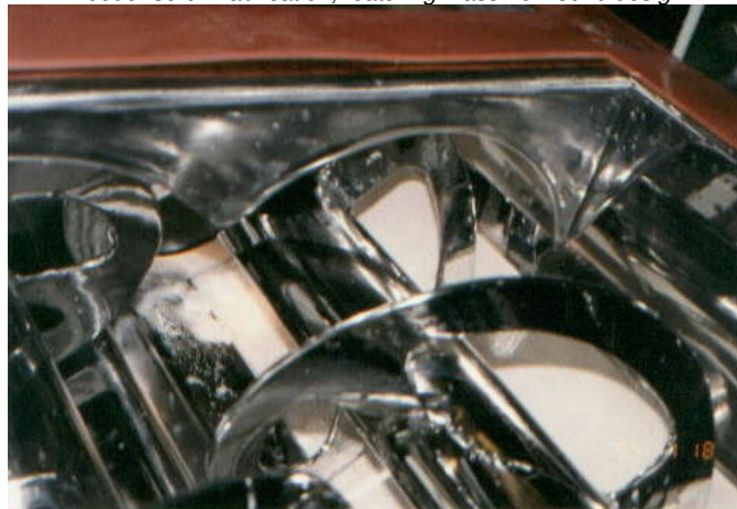
Polished ribbon feeder helix passing beneath shroud
