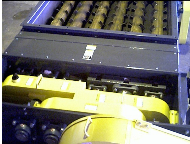
Model 0209-LBB-6-NS intermittent-spiral feeder for synthetic gypsum
