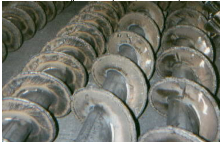
Weld-on hard facing treatment for abrasion resistance
