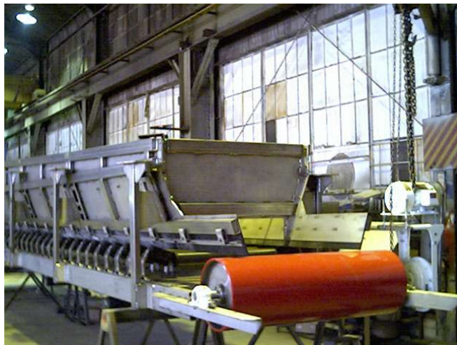
Stainless filter cake feeder belt with urethane pulley
