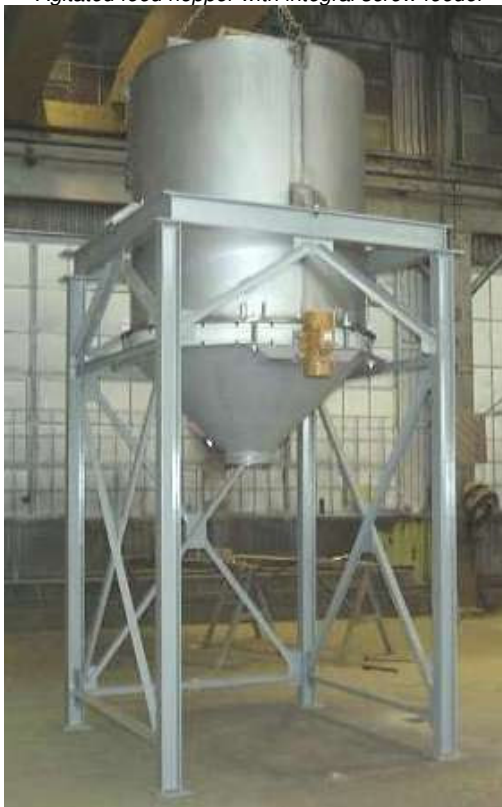
Stainless pack-out hopper with gyratory bin discharger and support structure
