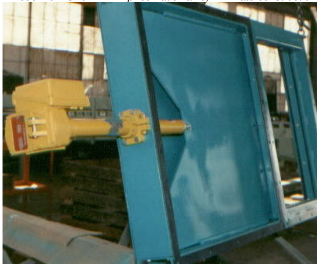
Modulating cam-roller gate valve with electric linear actuator
