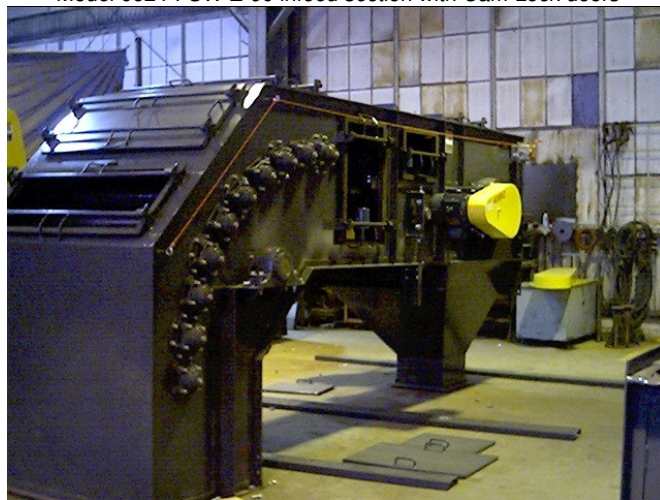
Horizontal discharge section with radius-curve roller assembly
