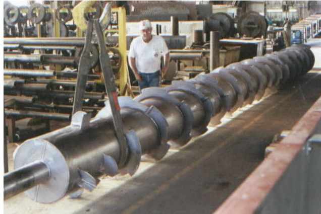
Engineered "LongSpan" conveyor helix @ ~ 40 ft.
