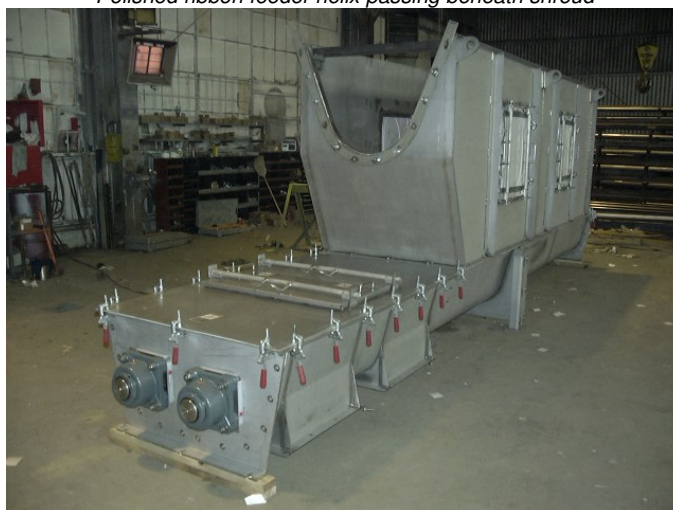
Stainless twin feeder with integral surge hopper
