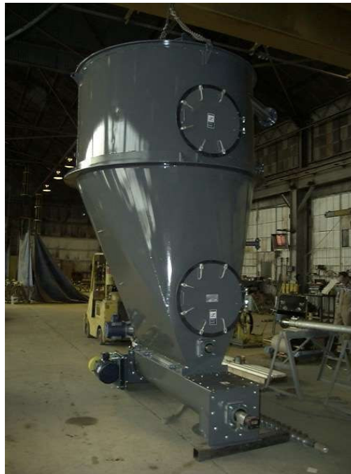
Agitated feed hopper with integral screw feeder
