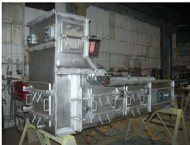
Model 0624-FSW-Z-90 infeed section with Cam-Lock doors
