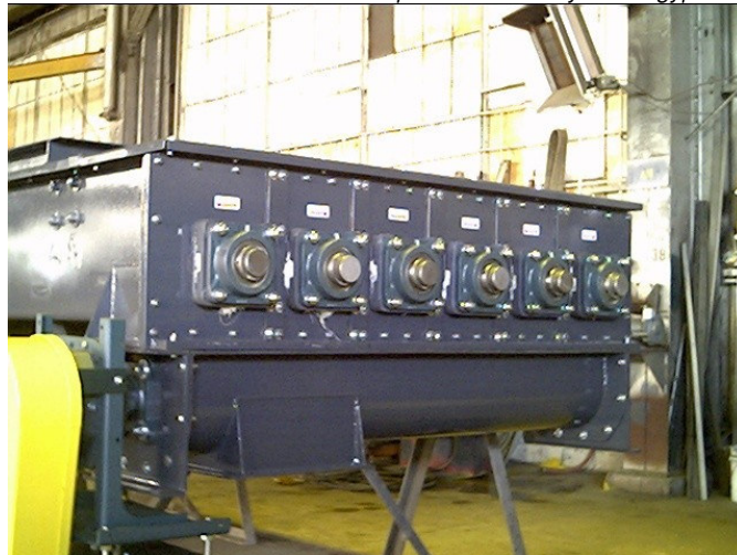
Six-screw bin bottom with integral collection screw conveyor
