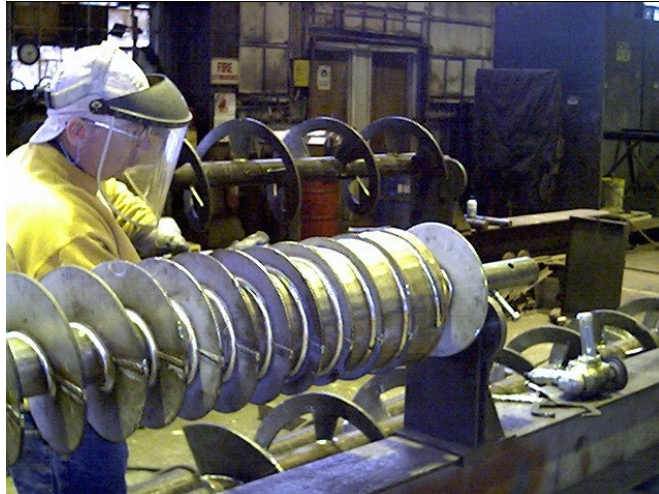
Feeder screw fabrication, featuring mass-flow cone design
