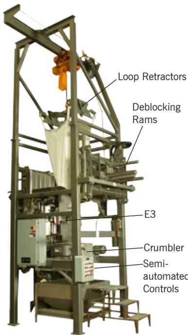
A single hardened block of material is reduced to lump sizes that will discharge out of the bag and is then further reduced to a pneumatically conveyable particle size.
