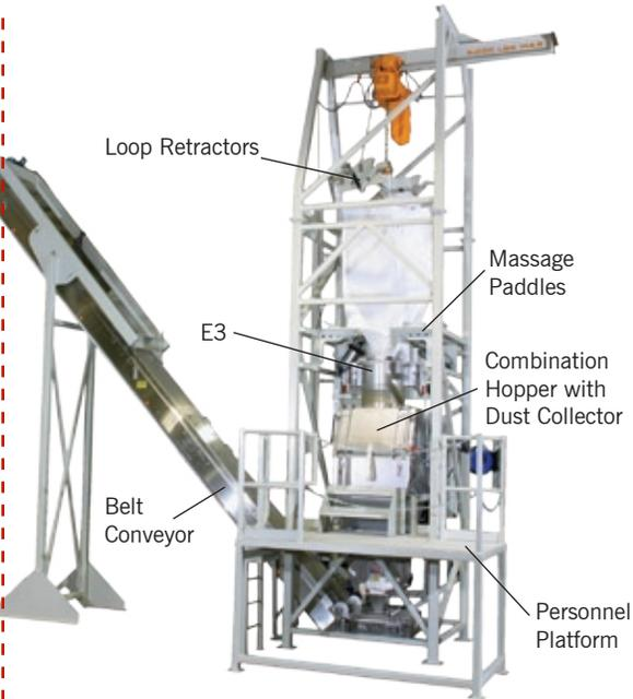
Dusty and agglomerated material supplied in bulk bags and 50 lb. bags are discharged from the bags and transferred through a screener into different containers in a dust free manner. The integral dust collector returns the captured dust directly back into the process.
