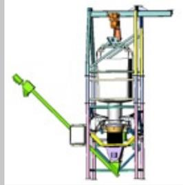
The foresight provided by the 3D model helps eliminate typical installation problems and hindsight wish lists. However, NBE goes one step further by fully assembling and testing the equipment with your material prior to shipping. This ensures the performance of the discharger within your system.
