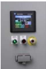
PLC controls automate a range of operations from simply starting and stopping material transfer conveyors, to automating the entire sequence of operations based on downstream
