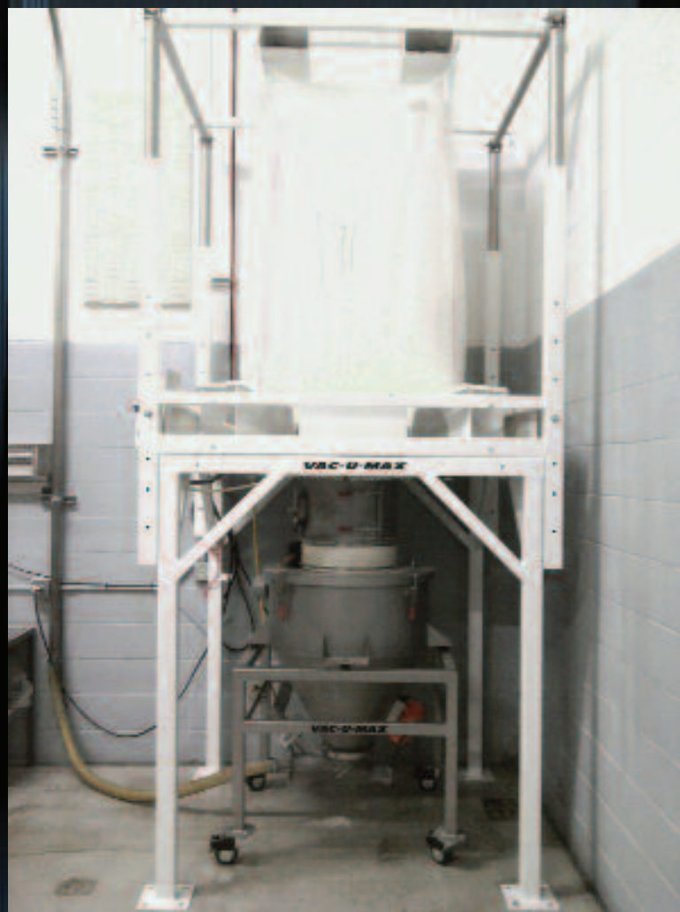
The custom-designed bulk bag discharger stand provides dust-free bulk bag unloading and is easy to clean around, improving the plant's sanitary conditions.
