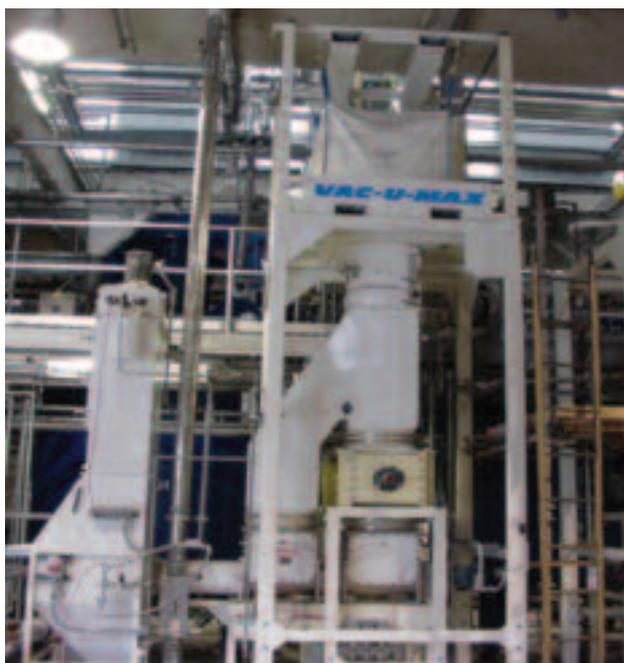
bulk bag assembly was over 20 feet high to accommodate the diverter valve. Bulk material was unloaded from bulk bags, with minor ingredients hand dumped via integrated reverse jet filter type bag dump station, fed via a screw feeder and on to the first of two Aero-mechanical conveyors.
